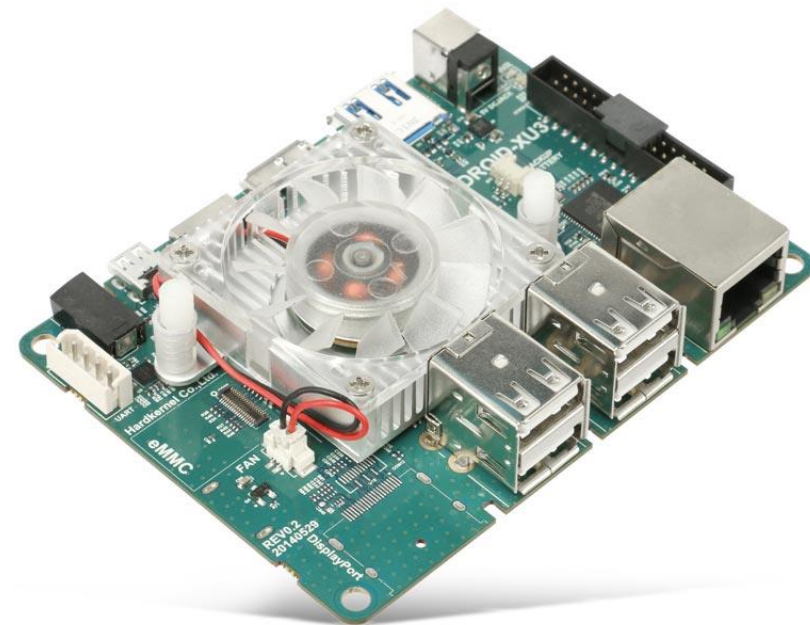
Odroid-XU3 board. Source: www.hardkernel.com
